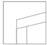
Now saw all parts and corners to the correct measurements. Size 1 and Size 4 come from the 4200mm F-profiles. Size 2 and size 3 come from the 2000mm F profile.
