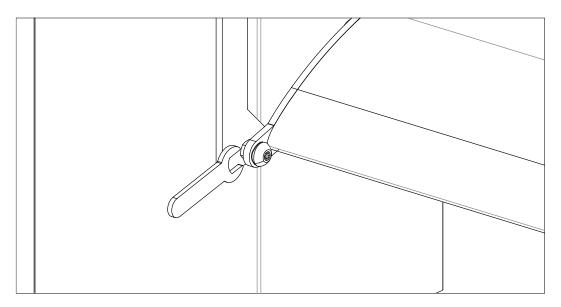
**Louvres turn too lightly:** you can make the louvres turn more heavily as follows. Dismantle the screw with the spring washer and nut. Then add an additional spring washer This process will not need to be done for all louvres. Adjust louvre after louvre, until you have achieved the desired result.
