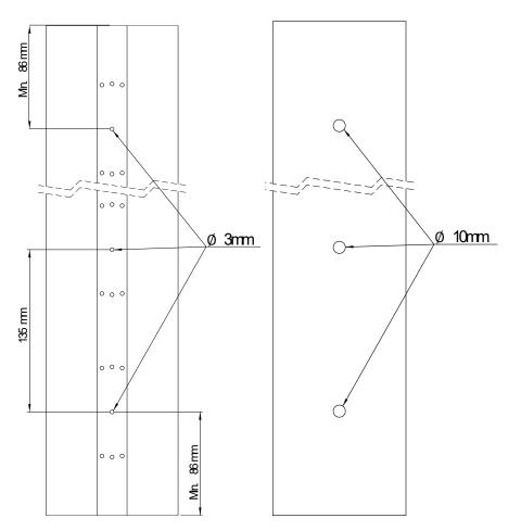
c. **Drilling the holes:** Remove the drilling jig and drill the pre-drilled holes through with a drill of Ø10 mm.
