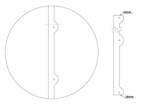
**b.** Connecting the connection rod: attach the connection rod to the louvres. Do this by screwing the screws, supplied with the installation kit, to the rod. Repeat this action for all louvres and on both sides.
