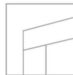
3. Saw the Grillo parts and top cover to length. The Grillo parts should be cut to  $(D) - 10\text{mm}$  and the top cover to  $(D) - 4\text{mm}$ .
