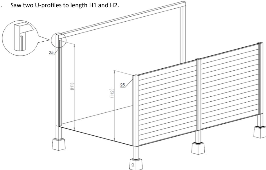
2. Install both U-profiles against the posts by screwing them against the posts from the inside (Let the sides of the U-profiles to run parallel with the sides of the posts). Place a screw every +/- 50 cm. Pre-drill first.
