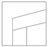
3. Place the first roofing sheet between the beams. **Note:** UV side up, the long condensation profile with the tab down and on the gutter side.
