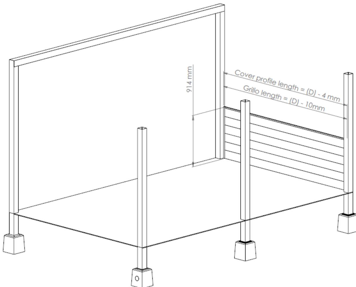
4. Place the Grillo parts 1 by 1 in the U-profile from above. The profiles click together with a little force. Finally, place the top cover. (Make sure you place the Grillo profiles properly, otherwise the top cover will not fit).
