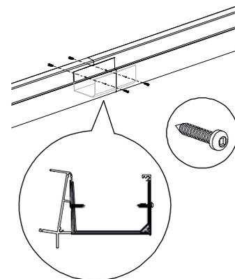
**6.** The gutter extension can now be secured with the short stainless steel screws in the chamber of the gutter and on the front side under the decorative profile. Put sealant on the assembly so it is smooth and waterproof!
