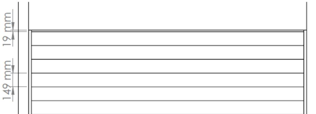
2. Install both U-profiles against the posts by screwing them against the posts from the inside. Pre-drill first.
