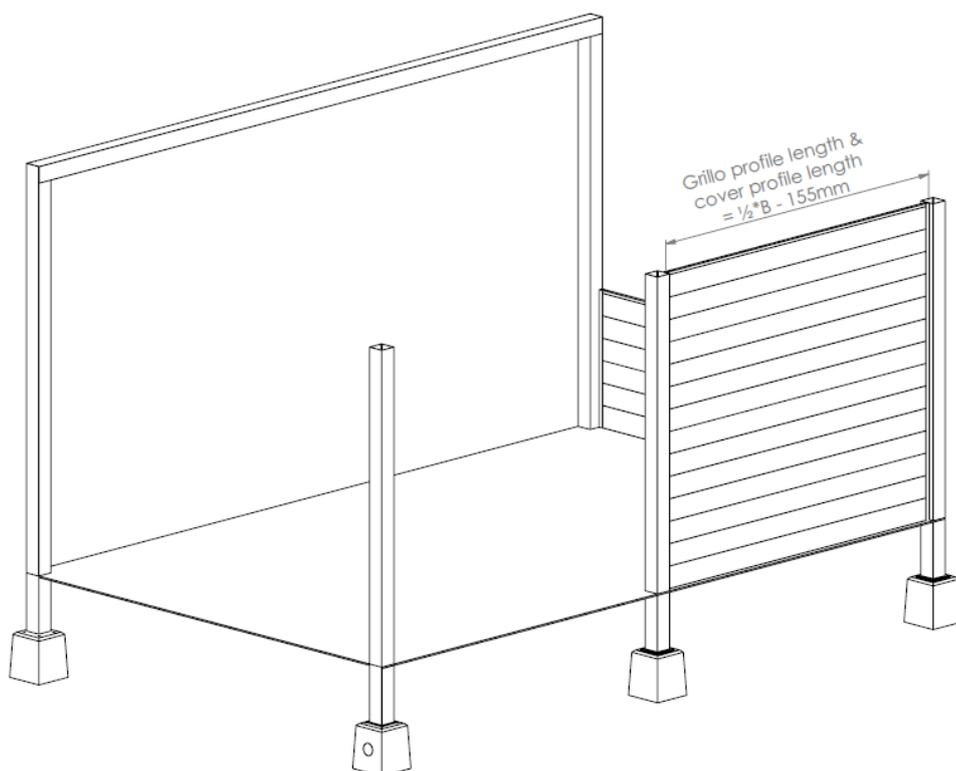
5. Connect the Grillo parts and the U-profiles with each other by screwing a few screws through the side wall of the U-profiled into the Grillo parts. Pre-drill first.
